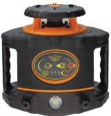
Place the instrument on a horizontal platform
